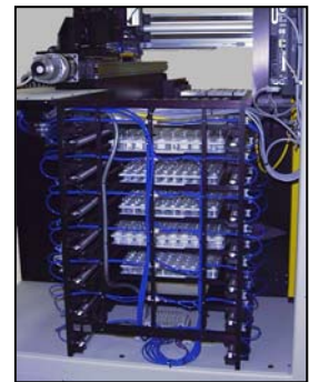
A hotel system is used to increase the capacity of the machine.
