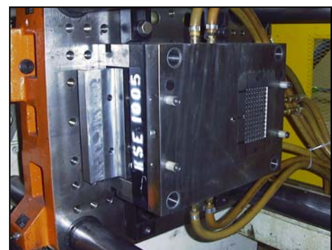
Injection mold tool in the press.
