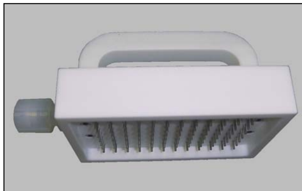
Solvent dispenser for multi-well apparatus. Withstands harsh chemical environments.
