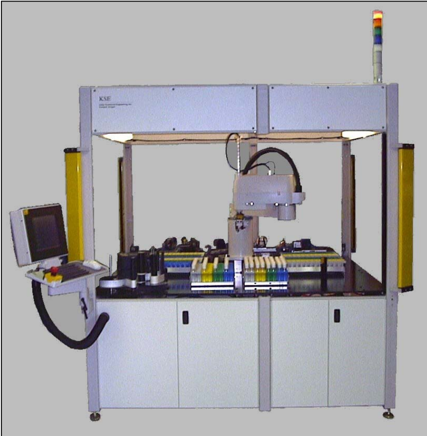
Fruit fly transfer machine, fully automated. Transfers live fruit flies from old vials to new vials with fresh food.
