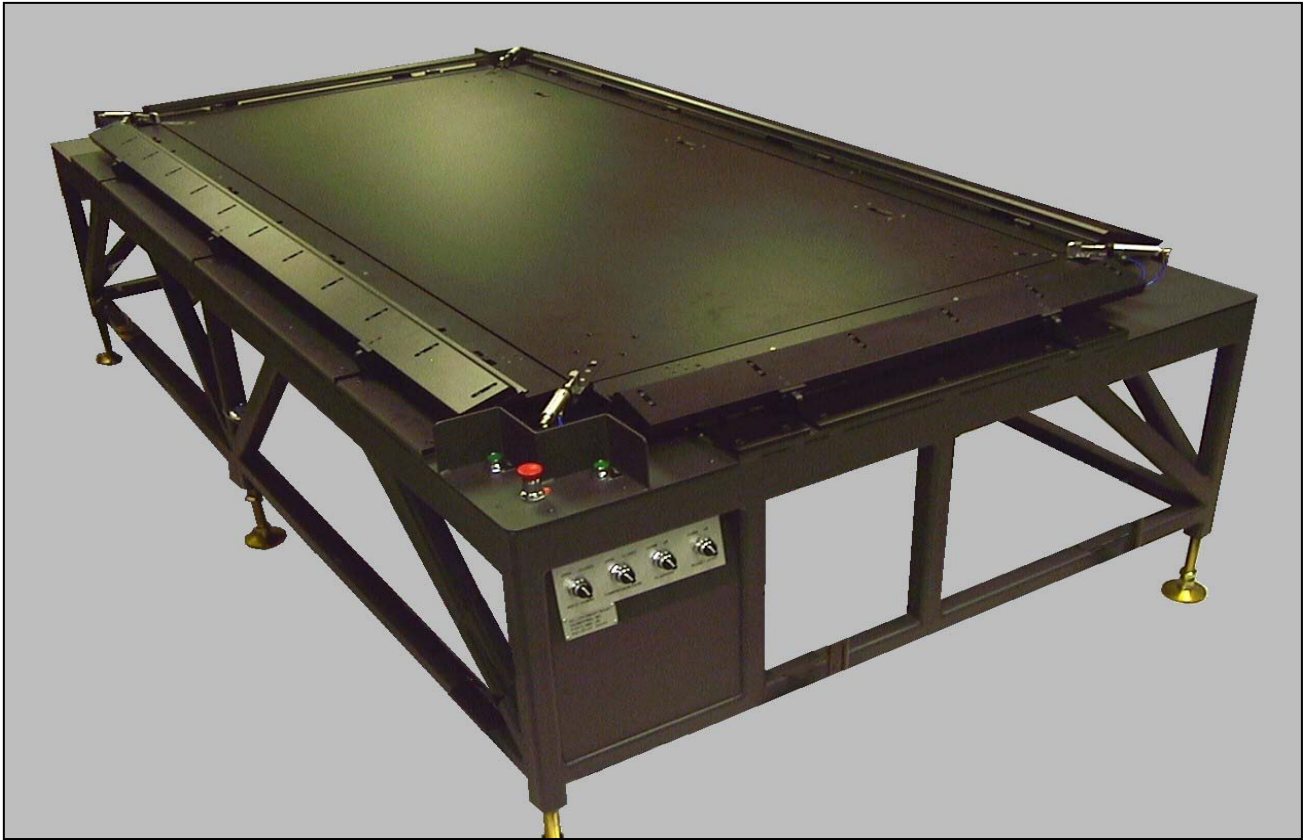
Assembly machine for computerized dry-erase boards. 100% pneumatically controlled. Shop air is all that is needed for operation.
