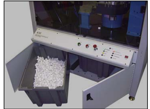
Crimped buzz plugs are deposited into a bin. A sensor signals operator when to empty the bin.
