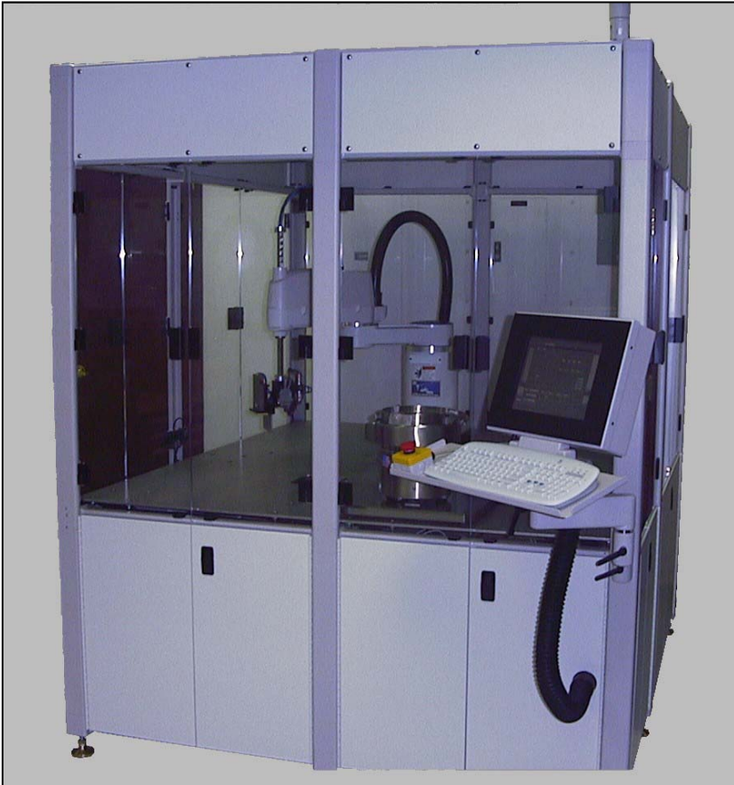
Hi-Speed Automated Machine inserts 9,000 components per hour into an assembly used in drug discovery and combinational chemistry.
