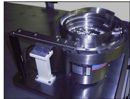
Vibratory bowl feeder presents the parts to the robotic end effector at high speeds.
